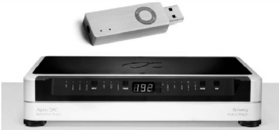
Fig.7-3 DACs range from simple plug-in devices to elaborate multi-input machines. (Courtesy Audioengine [top] and Berkeley Audio Design [bottom])
