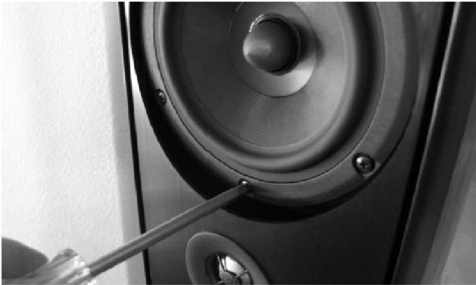
Fig.15-10 Periodically tighten the bolts holding the loudspeaker drivers to the baffle.
