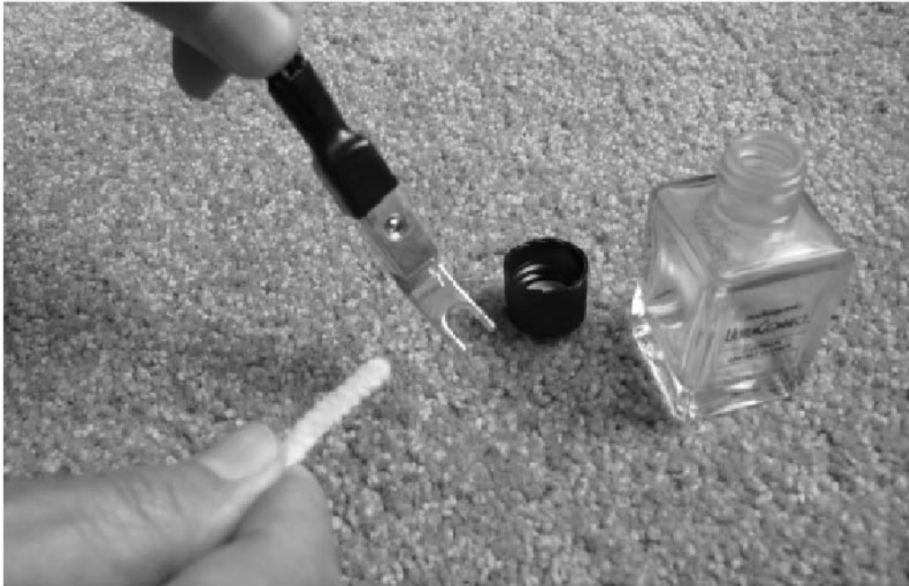
Fig.15-8 Periodically clean spade lugs, binding posts, RCA plugs, RCA jacks, XLR jacks, XLR plugs, tube pins, tube sockets, and other connections with contact cleaner.
