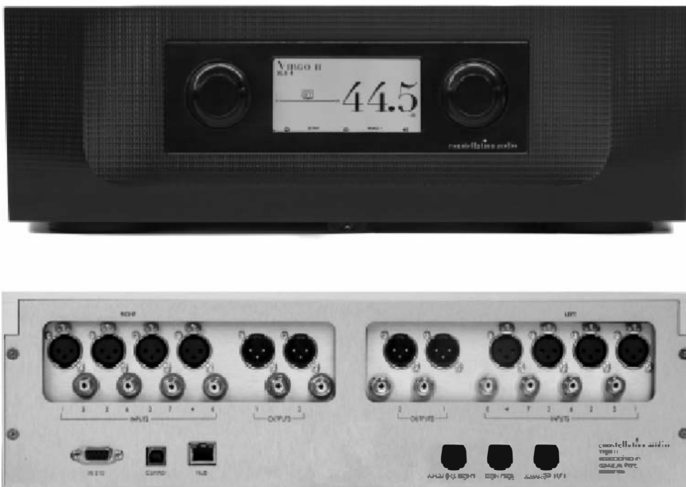
Fig.4-4 A line-stage preamp’s front and rear panels. (Courtesy Constellation Audio)
