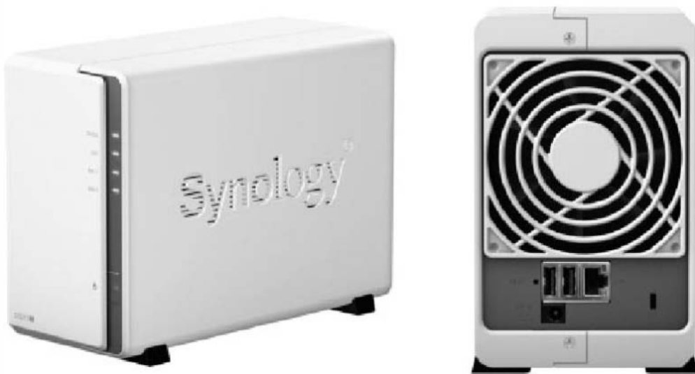
Fig.8-6 A dual-bay NAS drive designed for networked media (Courtesy Synology)
