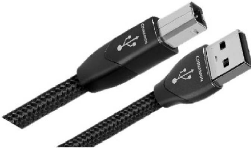
Fig.7-6 A USB cable for audio has a Type A connector on the end that connects to a computer (lower image) and a Type B connector on the end that connects to the DAC (upper image). (Courtesy AudioQuest)
