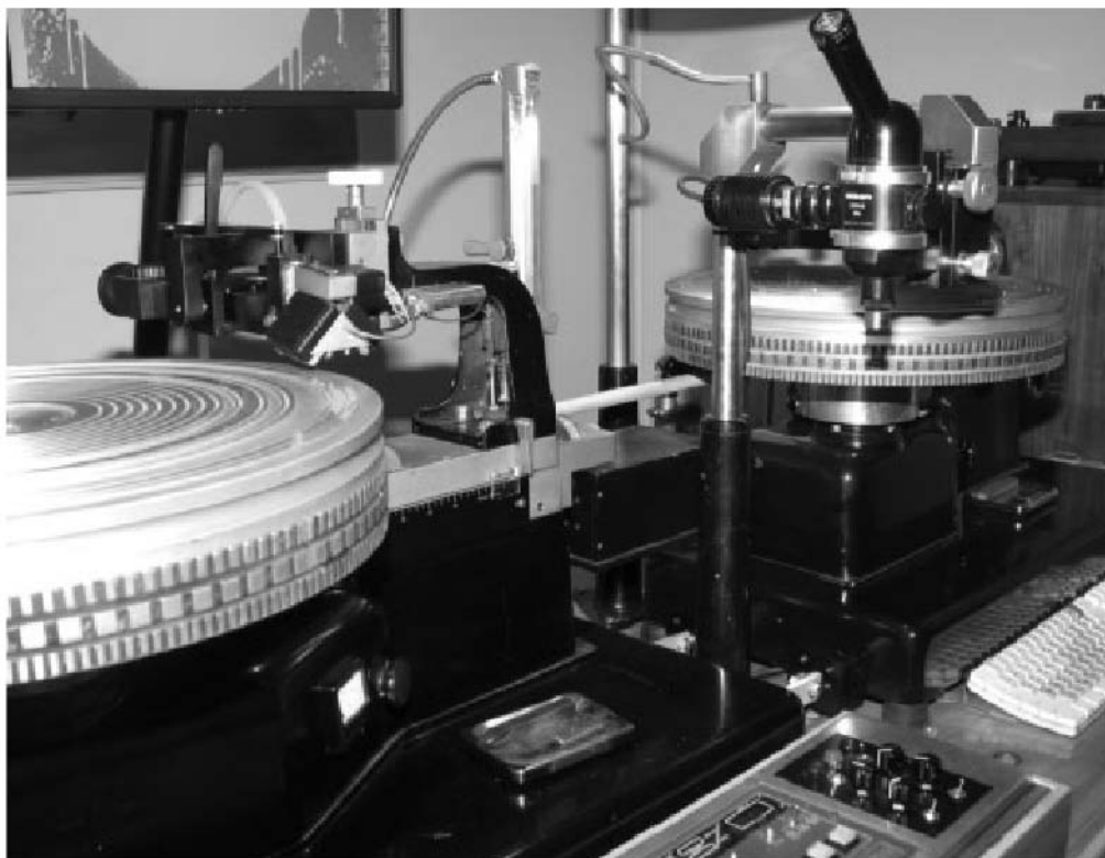
Fig.9-15 A pair of LP mastering lathes. (Courtesy The Mastering Lab; photo by Neil Gader)
