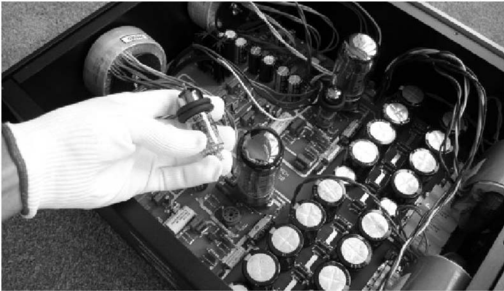
Fig.15-9 Wear gloves when installing or replacing vacuum tubes. Note the tube dampers, the two black rings surrounding the tube.
