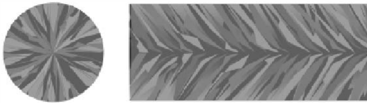
Fig.10-5 Copper in cables and interconnects has a grain structure. (Courtesy AudioQuest)
