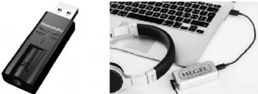
Fig.13-13 A portable DAC and headphone amp can plug directly into your computer's USB port (left), or via a USB cable (right) (Courtesy AudioQuest [left] and Hegel [right])
