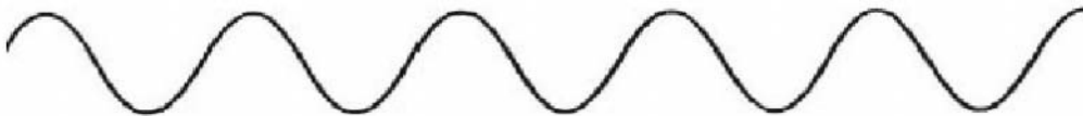
Fig.B-7 The 120V, 60Hz AC from a wall socket is a sinewave.
