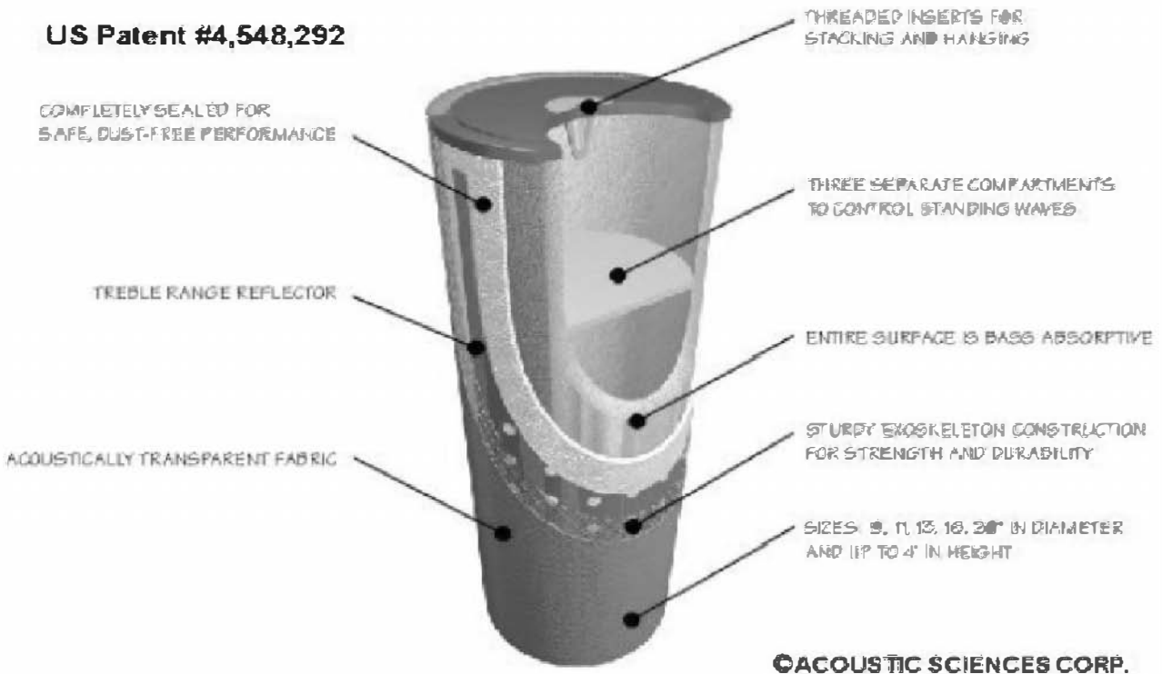
Fig.14-20 Tube Trap construction (Courtesy Acoustic Sciences Corporation)
