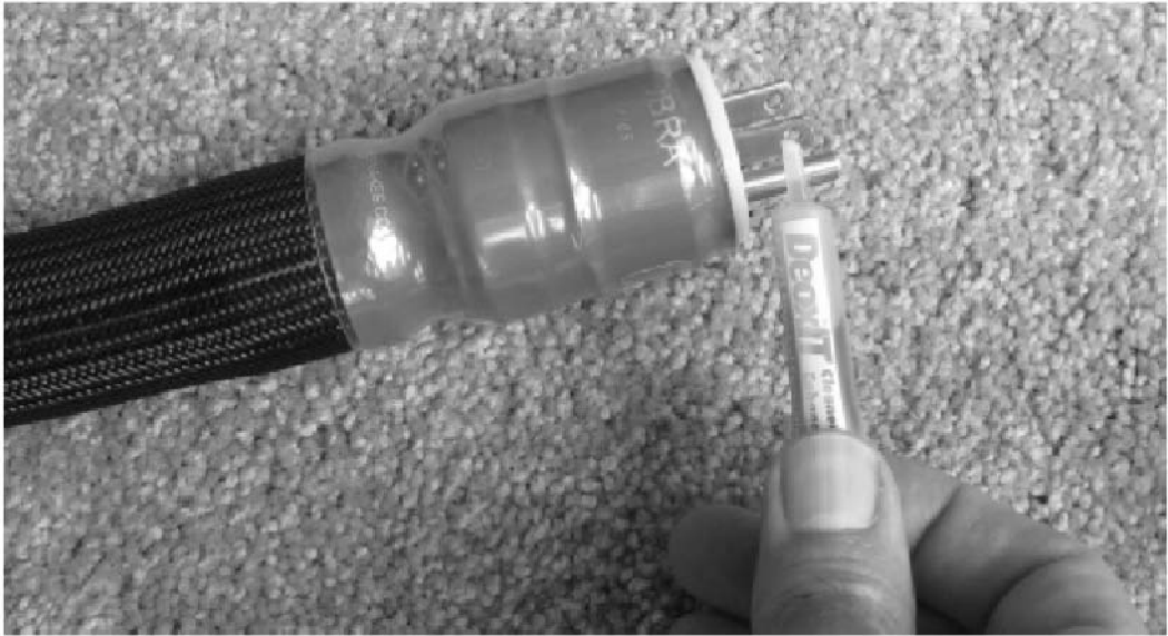
Fig.15-1 Applying contact enhancer to the blades of AC cords is a simple and effective tweak.
