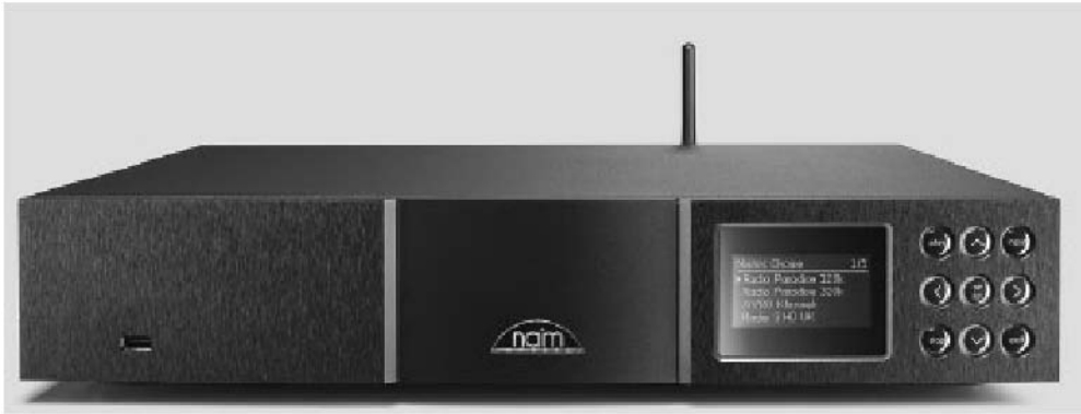
Fig.8-4 A network-capable DAC that can become a full-fledged music server. (Courtesy Naim Audio)
