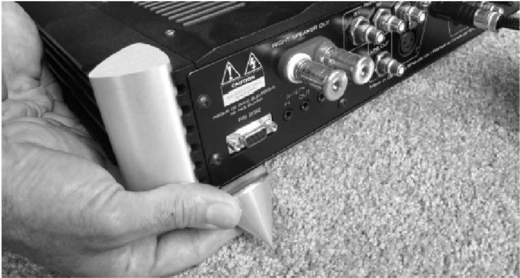
Fig.15-6 Spikes or cones beneath an amplifier or integrated amplifier on a carpeted floor help damp vibrations and provide much-needed ventilation.
