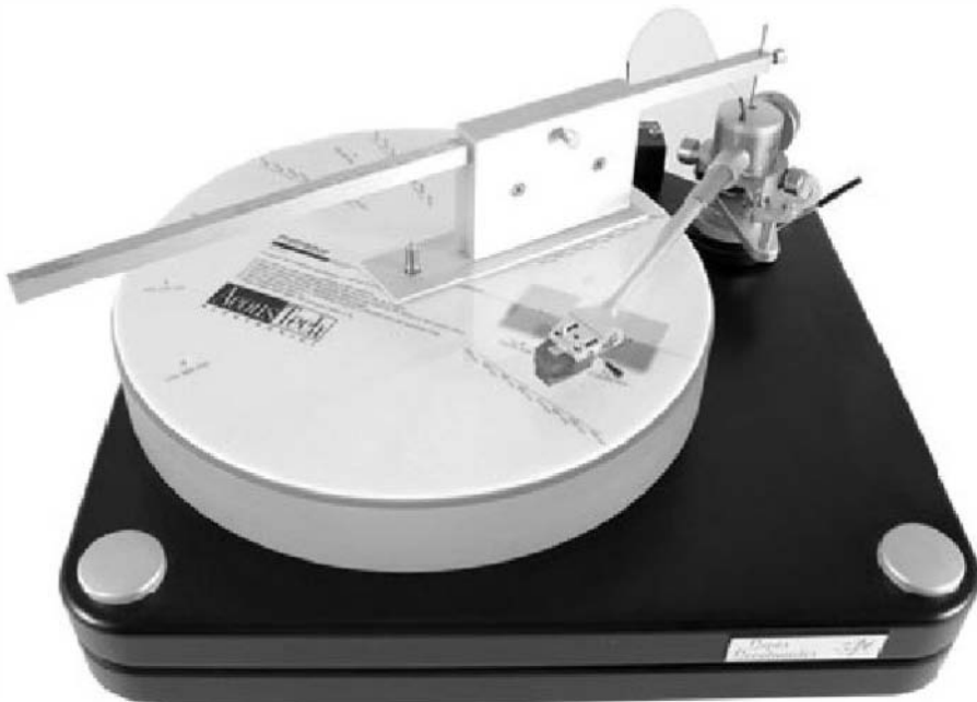
Fig.9-11 A high-quality protractor allows you to optimally set up your tonearm and cartridge. (Courtesy Dr. Feickert Analogue and AcousTech)
