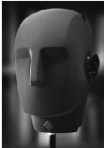
Fig.13-9 Binaural recordings are made with microphones inserted in the “ear canals” of a dummy head. (Courtesy Georg Neumann)
